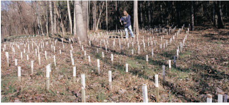
The effectiveness of preservatives at various retentions in different species is evaluated using test stakes.
